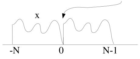
To avoid such artifactual frequency content one should "window", i.e. multiply the time signal with a windowing function that makes a smooth transition.
